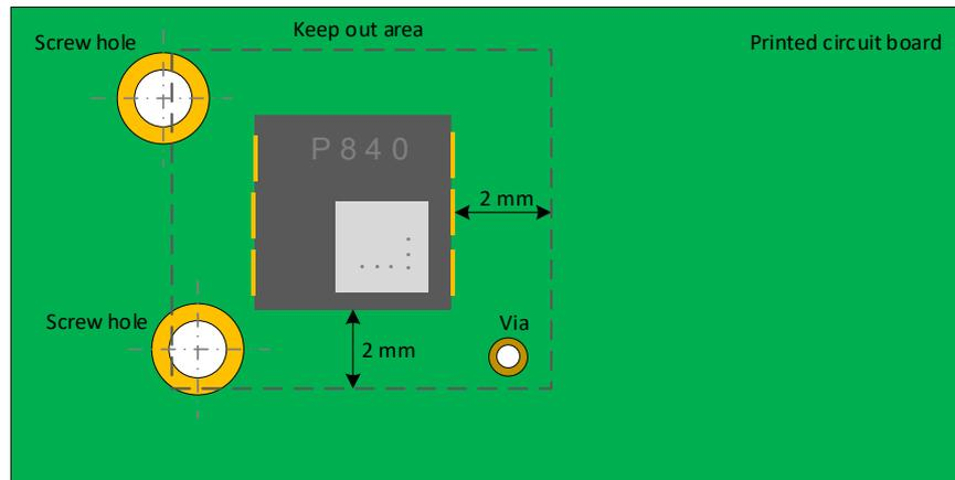
Figure 4: Components inside sensor keep out area
