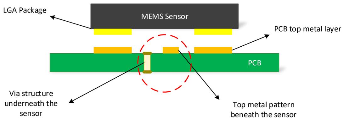
Figure 2: Incorrect PCB design
