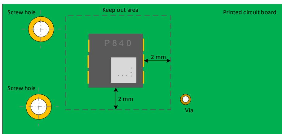
Figure 5: Components outside sensor keep out area
