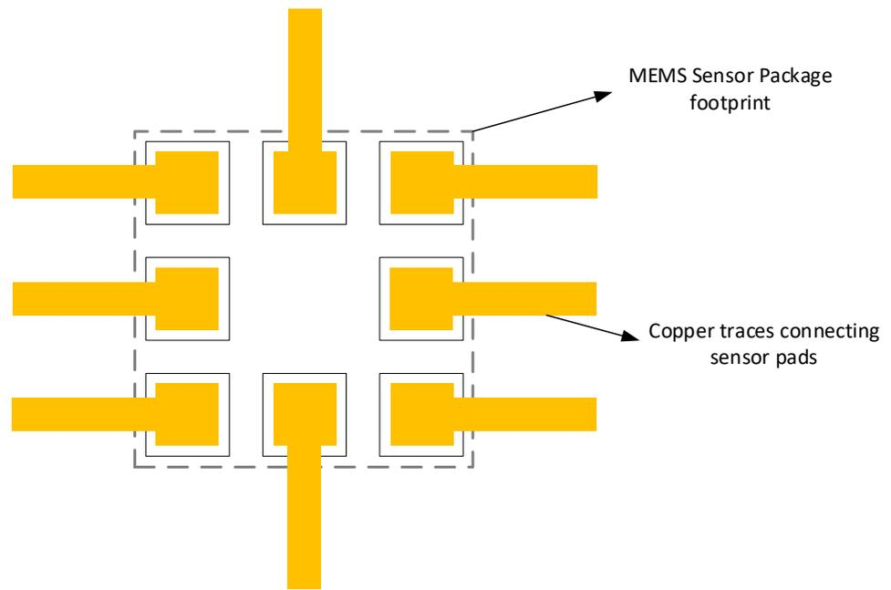
Figure 7: Symmetrical trace and sensor pad connections
